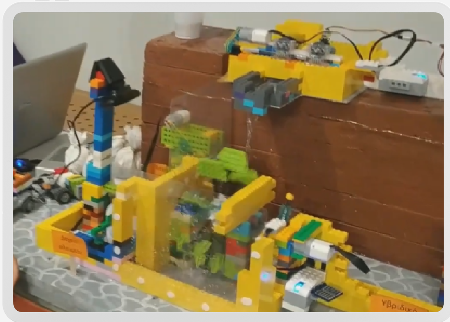
Hybrid watermill. The camera measures the rotation speed of the mill. The water flow is regulated according to the speed of the mill.
